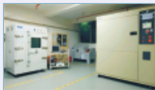
Faster temperature chamber & Thermal Shock Test Chamber
